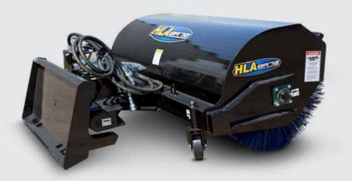
The hydraulic rotary broom comes ready with everything you need including hydraulic hoses, flat-faced couplers, and an electric selector valve and wire kit. Hooked up and ready to go the brooms direct motor drive requires 12-20 GPM of hydraulic flow to turn the 26" diameter poly/steel wafers.
